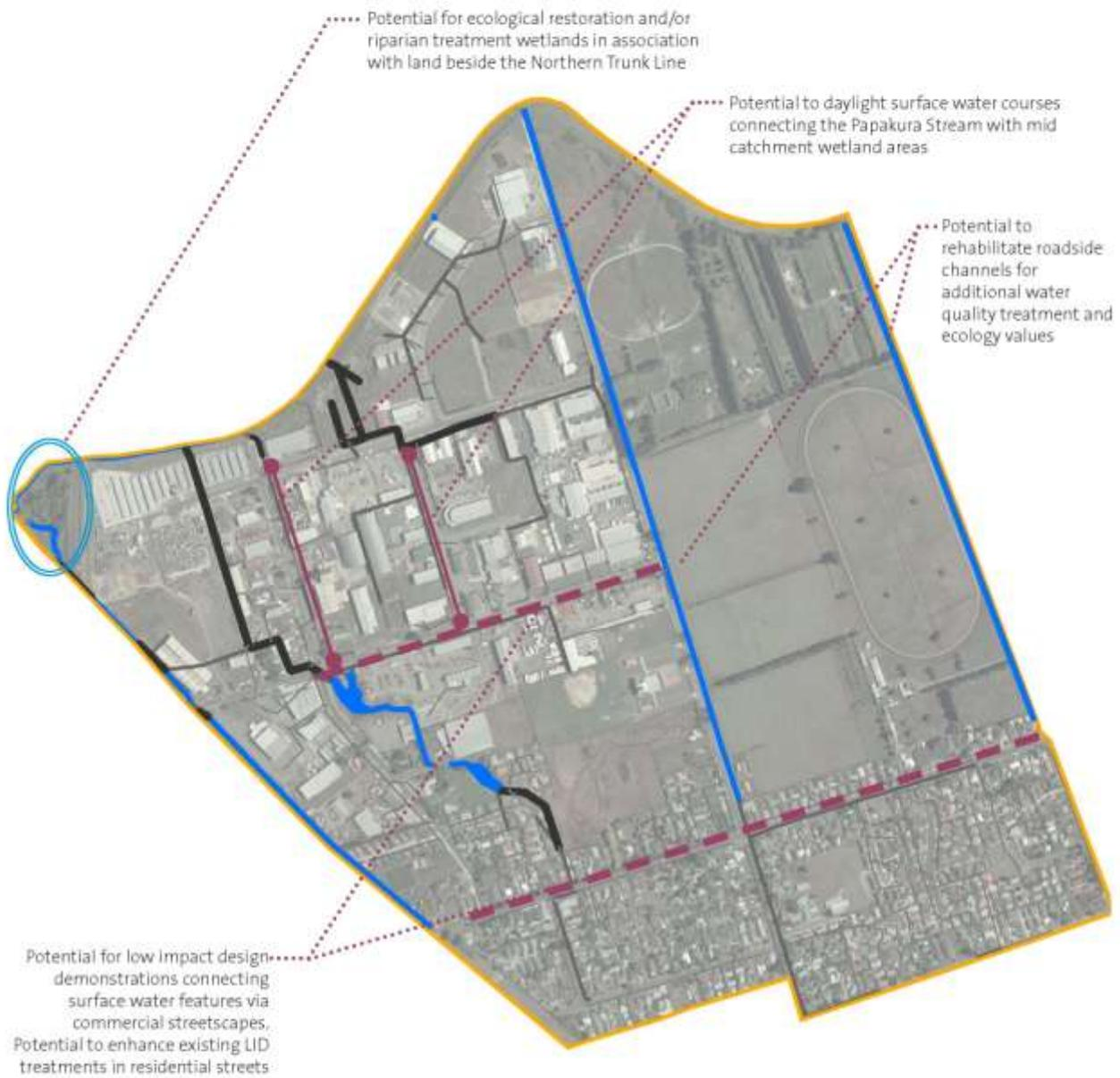
Papakura SW Catchment boundaries are based on District Council stormwater sub-catchment boundaries where they coincide with reticulated flows directed to the Papakura Stream. This excludes reticulation directly to the Pahurehure Inlet. Subcatchment boundaries relating to overland flows are based on Boffa Miskell LIDAR interpretation.
